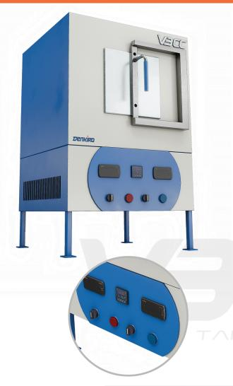
Compact Design: Space-saving dimensions ranging from 150 x 150 x 150 mm to  $300 \times 300 \times 300$  mm, offering versatility to accommodate various sample sizes and quantities.
